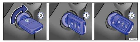
Fig. 103 In the ignition switch: Vehicle key positions.
