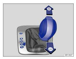
Fig. 113 Selector lever in Tiptronic position.
