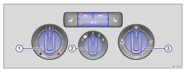
Fig. 123 In the center console: Manual AC controls.
