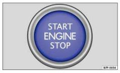
Fig. 104 In the center console: Starter button of the Keyless Access locking and starting system.
