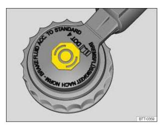
Fig. 115 In the engine compartment: Brake fluid reservoir cap.
