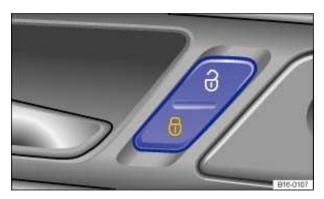
Fig. 21 In the driver and front passenger doors: Power locking button.
