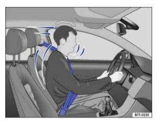
Fig. 49 Belted driver secured by the correctly worn safety belt in the event of a sudden braking maneuver.
