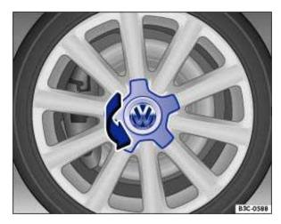
Fig. 160 Twisting the hubcap off.
