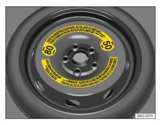
Fig. 143 In the luggage compartment: Compact spare wheel.
