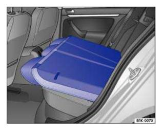
Fig. 83 Rear seat bench: Seat backrest folded down.
