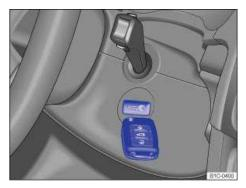
Fig. 105 Emergency starting feature on vehicles with Keyless Access.
