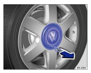
Fig. 159 Pulling the hubcap off.
