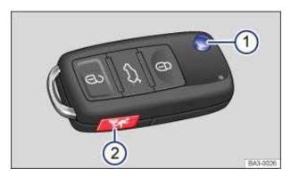
Fig. 16 Remote control vehicle key with panic button.
