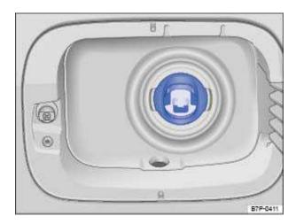
Fig. 129 With open fuel cap: Misfueling guard in the fuel filler neck.
