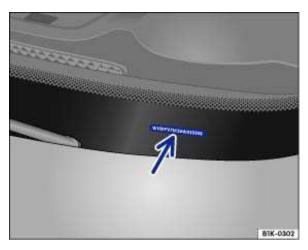
Fig. 15 Vehicle identification number (VIN).
