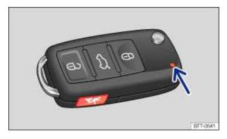
Fig. 17 Indicator light in the remote control vehicle key.
