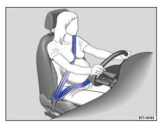
Fig. 53 Proper safety belt positioning for expectant mothers.
