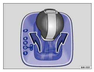
Fig. 155 Removing the selector gate cover.
